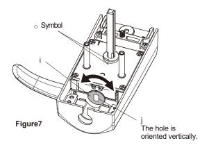
4. With the cylinder head (a) facing upward, insert it into the connecting part (i) (see Figure 8).
