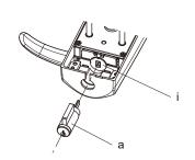
5. Rotate the cylinder (a) to the right (see Figure 9).
